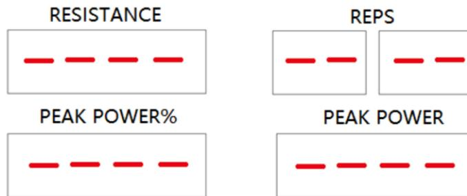
3.2.2 The frequency data cannot change normally during exercise: the position sensor is faulty.
